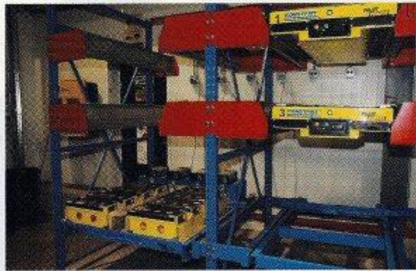
SPACE SAVINGS: The Pallet Runner carts run on rails attached to the 24 pallet deep rack structure. Only one aisle is required to reach pallets within the system.
